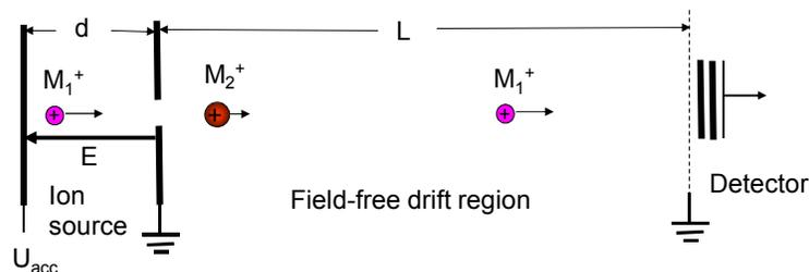
$$t_{of} = t_{delay} + t_{acc} + t_{drift} \quad (1)$$
