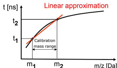
For a sufficiently narrow mass range, a linear approximation of  $t_{of}$  may be sufficient in terms of calibration accuracy (2 known calibrant masses are required here). However, for the calibration of an extended mass range, a quadratic polynomial provides a much better description of the relationship between flight time and  $m/z$ . Minimum 4 known calibrant masses are required when applying a quadratic calibration function!
